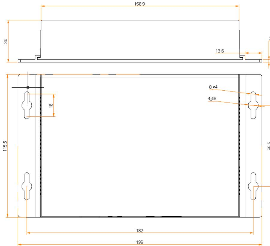
Tolerance:  $\pm 0.3$  Unit: mm
