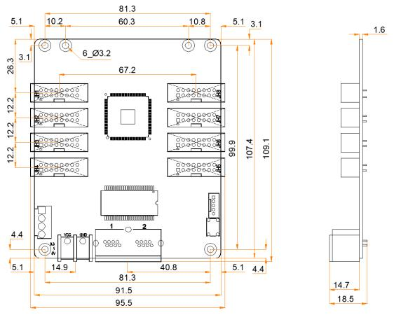
Tolerance: ±0.3 Unit: mm
